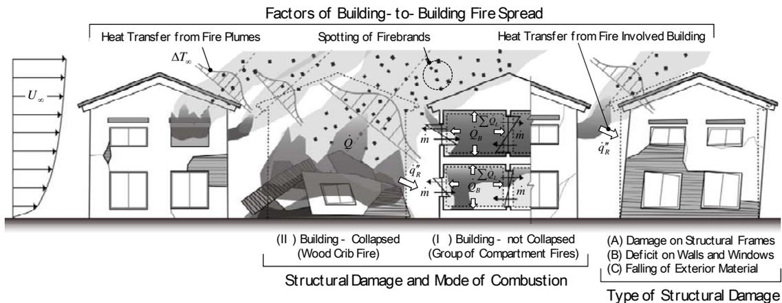
Fig.1. Schematic of the post-earthquake fire spread model.
