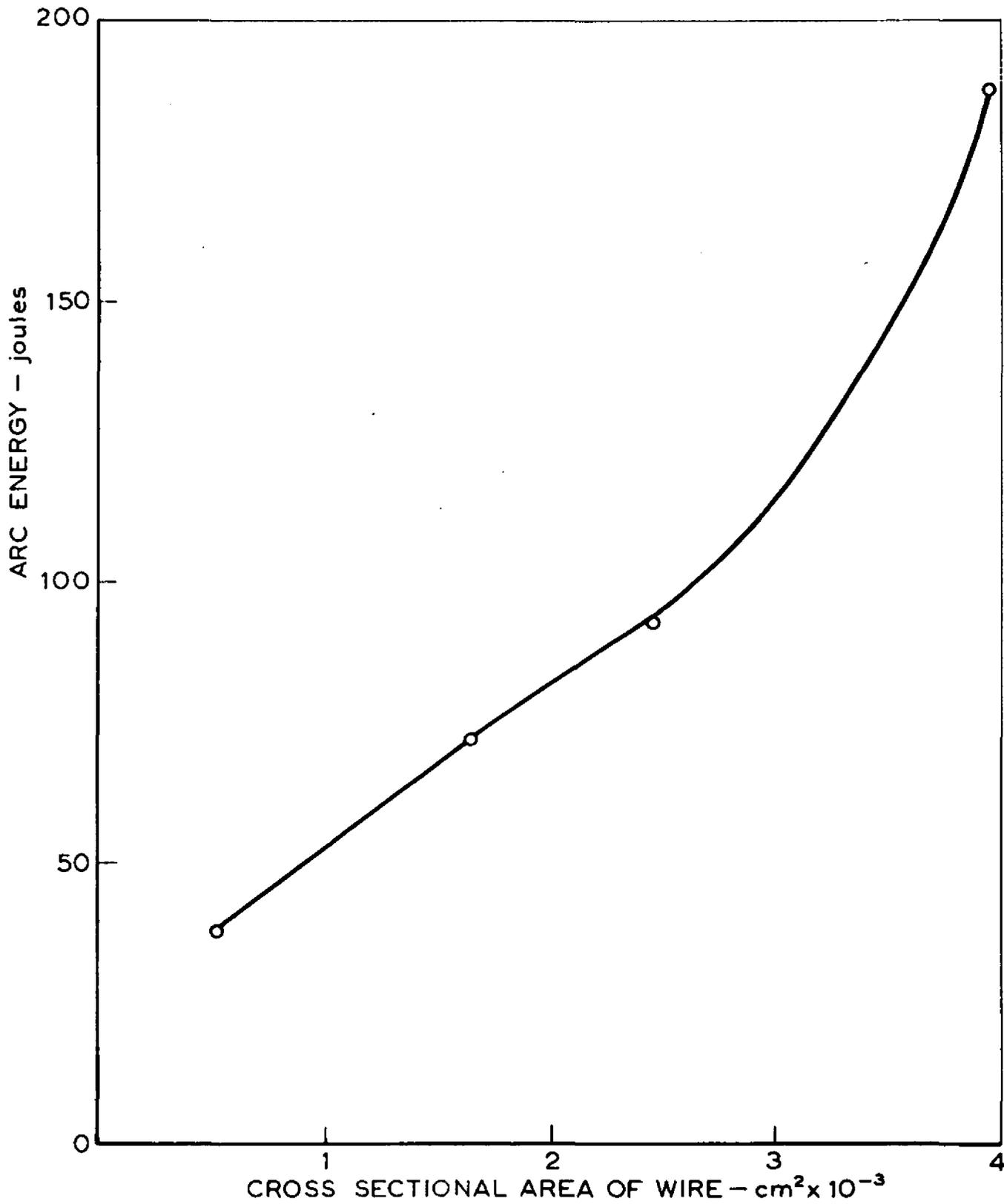
FIG. 5. RELATION BETWEEN THE THICKNESS OF WIRE AND ARC ENERGY
