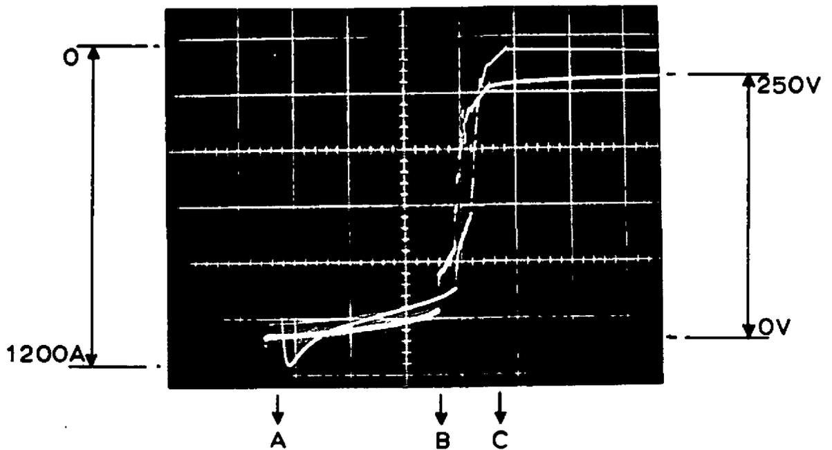
FIG.3. OSCILLOSCOPE RECORD OF VOLTAGE AND CURRENT WHILE FUSING 0.07cm DIAMETER (22 SWG.) COPPER WIRE AT A PROSPECTIVE CURRENT OF 1200 A
