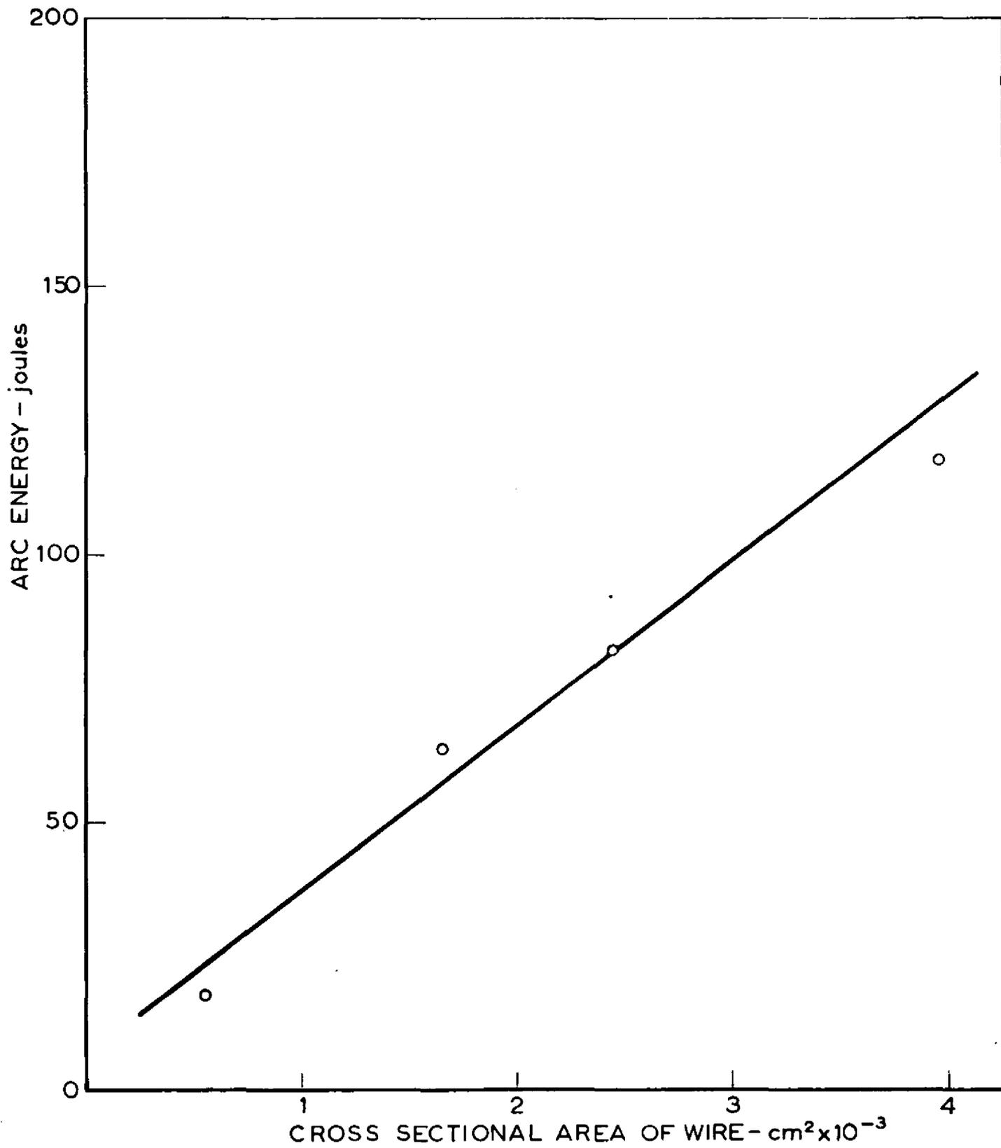
FIG. 4. RELATION BETWEEN THE THICKNESS OF WIRE AND ARC ENERGY
