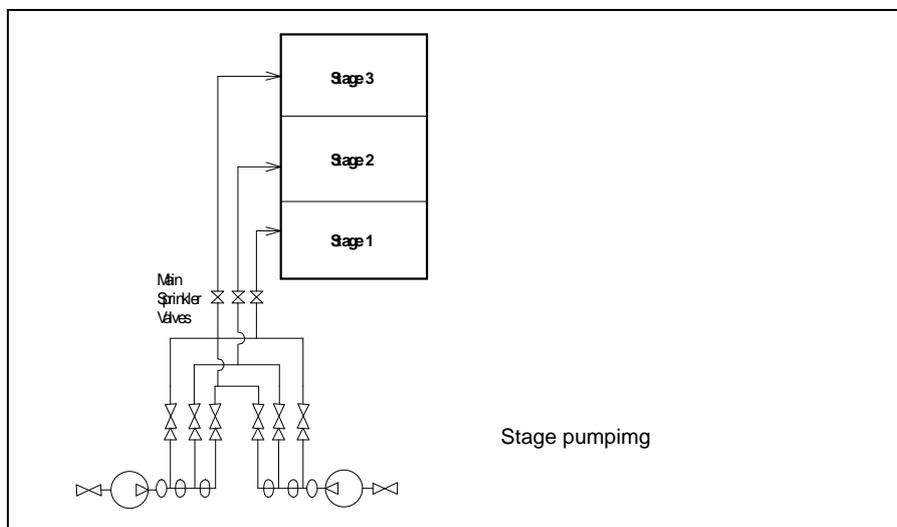
**FIGURE 2.** Water supply arrangement for upfeed system with multi-stage pumps
