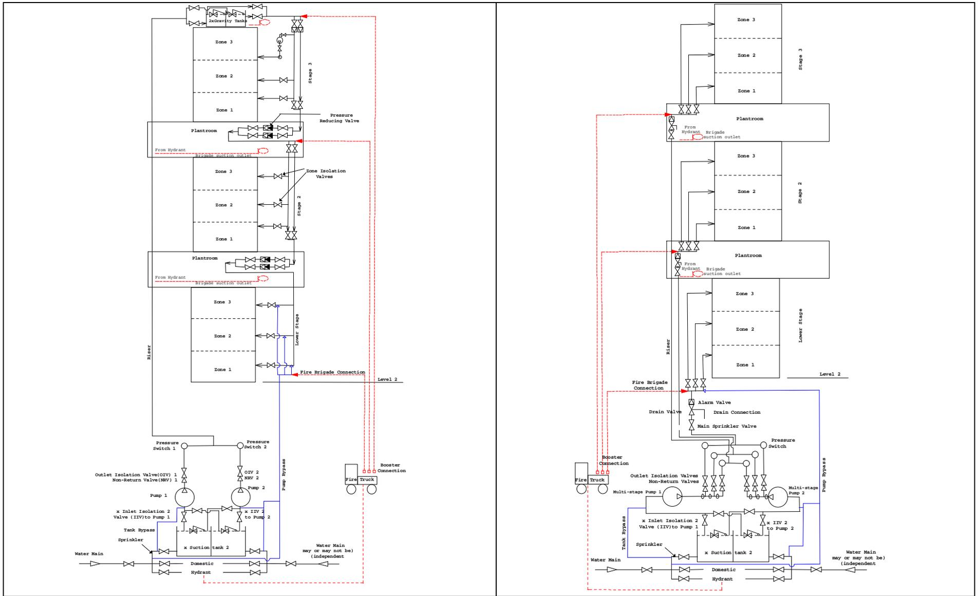
**FIGURE 3.** Details of water supply and sprinkler system for 60 storey building: (Left) Downfeed and (Right) Upfeed
