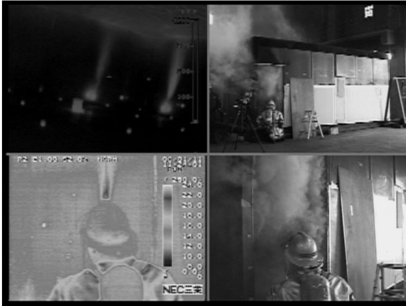
(a) Test 1. The fire room is filled with smoke and visibility is zero. Firefighter scans inside of the fire room through the opening. Locations of smoke candles and cups are identified.
