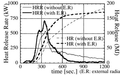
Figure 11. Difference of heat release rate of the low back chair without armrest 1 caused by external radiation
