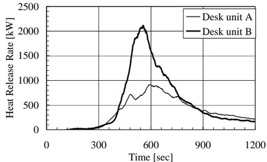
Figure 4. Heat release rate for Desk unit A and B
