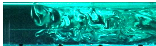
(c) supply ventilation rate= 117.8 liter/min·m
