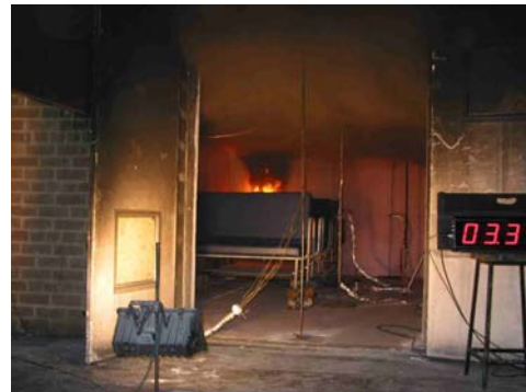
Figure 2. Seat experiment in progress showing hood
