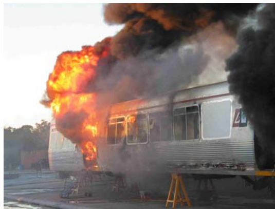
Figure 4. Full-scale fire test of single carriage (internal only)
