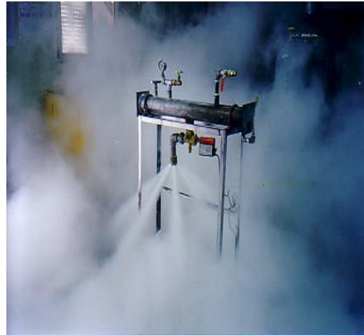
① Injection amount 11kg, Orifice10mm Set temperature 20°C, about 8 sec after discharge starts
