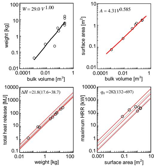
Figure 13 Survey Results (Trash)
