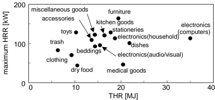
Figure 17 THR and maximum HRR values for the items with volume of 0.01m³
