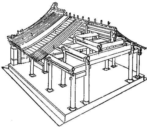
**Figure 1:** The wood structural frame of historical buildings in China.
