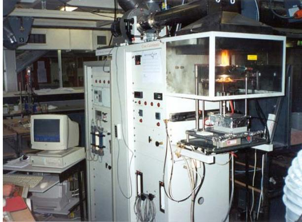
**Figure 1:** Cone Calorimeter.
