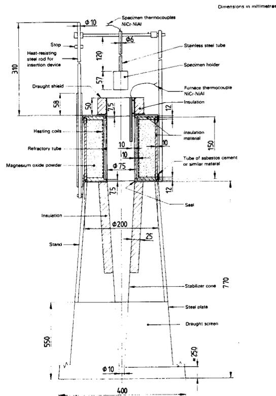
Fig. 1. Apparatus for testing non-combustibility according to EN ISO 1182
