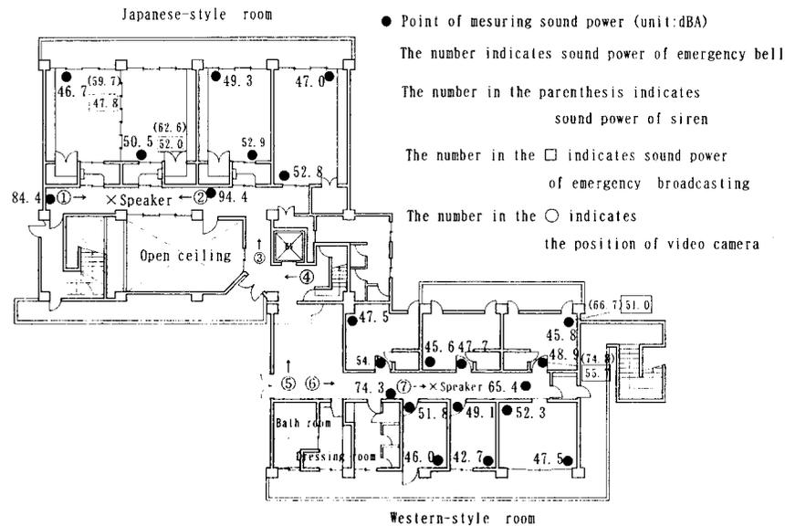
FIGURE 2. Plan of training at midnight be done and the result of measure sound power
