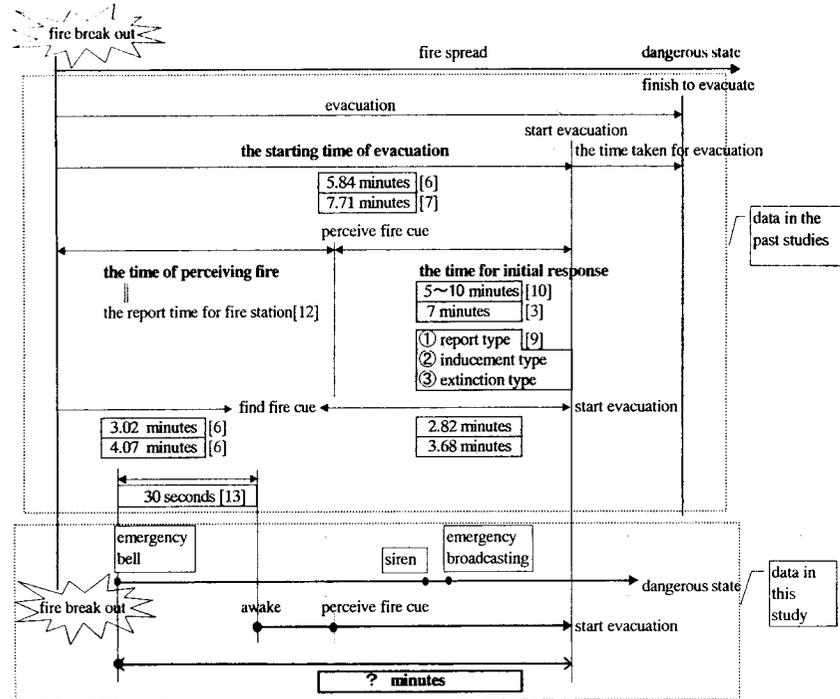
FIGURE 1. The relation between fire spread and evacuation
