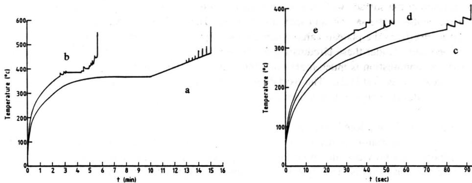
**Figure 2.** Typical temperature-time records for Mahogany samples at (a) 15.4; (b) 19.7; (c) 24.0; (d) 28.7; and (e) 31.7kW/m<sup>2</sup>.
